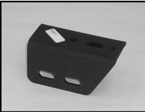
16955-11 (2) Rear lateral compression arm mounts
