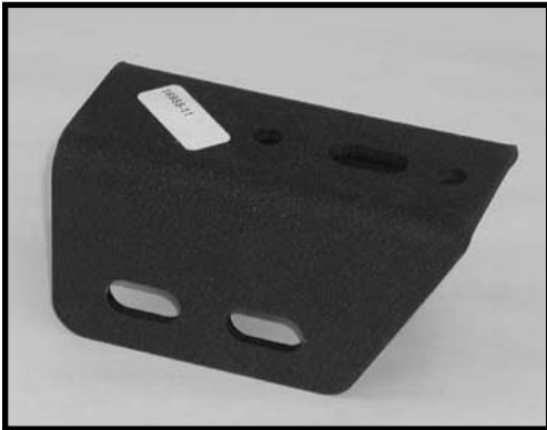
16955-11 (2) Front lateral compression arm mounts
