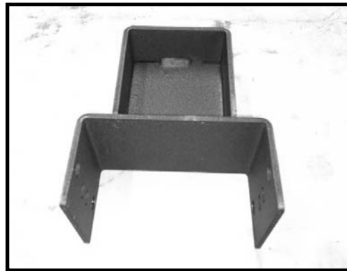
16085-18 (2) Rear bump stop extension brackets
