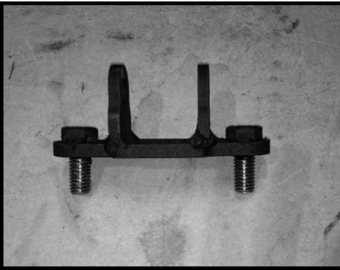
16085-15 (2) Upper shock relocation bracket
