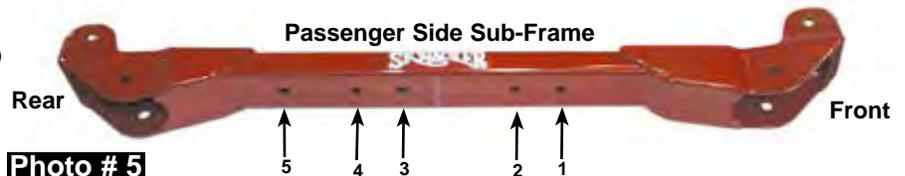
13. With the new Skyjacker sub frame attached with the lower bolts, drill the outer mounting locations using a 1/2" drill bit. Drill completely through the frame & the mounting tab located on the back side of the sub frame. (See Photo # 6) Once drilled, install the 1/2" x 4" fine thread bolt, washers, & nuts.
