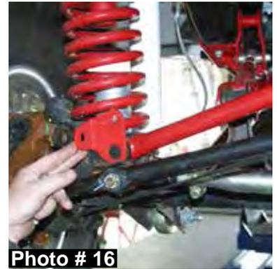
25. Install the frame end of the new Skyjacker track bar by following the hardware pictured. (See Photos # 17 & # 18) Being sure to keep the rod end square (parallel) with the frame mount. **Note:** Be sure no more than 1/2" of threads are extended from the bar (including the jam nut). Hold the rod end in place with a crescent wrench & tighten using a pipe wrench or crescent wrench on the jam nut.
