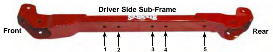
**Note:** Skyjacker sub frames are designed to work on 1997-2006 Jeep TJ's. Therefore, each sub frame will have multiple mounting holes.
