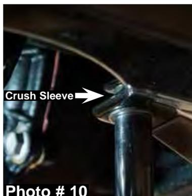
28. If equipped, install the OEM rear skid plate at the front mounting locations using the supplied crush sleeves, 8mm x 40mm bolts, & washers.
