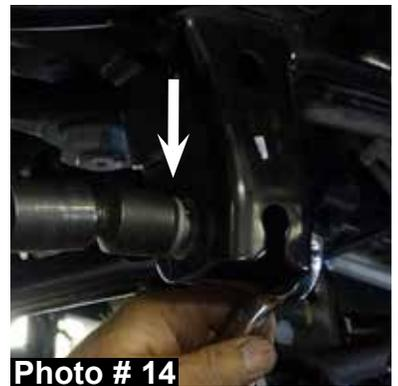
28. Using a measuring tape, check the front of the vehicle to make sure the body is centered over the front tires / wheels & adjust the new Skyjacker rod end to align with the lower track bar mounting location.
