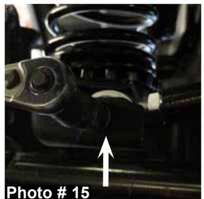
30. Tighten the supplied jam nut of the new Skyjacker adjustable front track bar using a 1 1/8" wrench.
