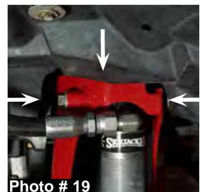
41. Assemble the new Skyjacker sway bar end links using the supplied steel sleeves, eyelets, & 1/4" snap pins. Install the new sway bar end links to the differential using the OEM hardware & to the OEM sway bar using the supplied 1/2" x 2 1/2" button head bolts, washers, nuts, & a 3/4" socket / wrench. (See Photo # 20)
