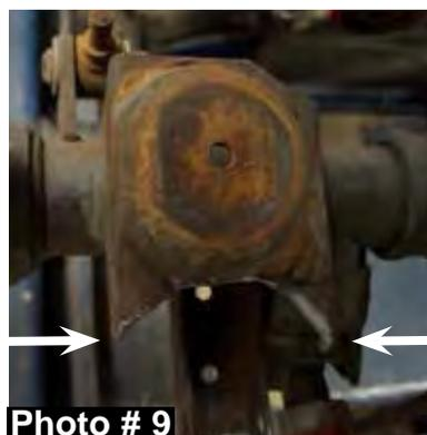
22. Clean up any imperfections & round any sharp edges using a grinder or similar tool.
