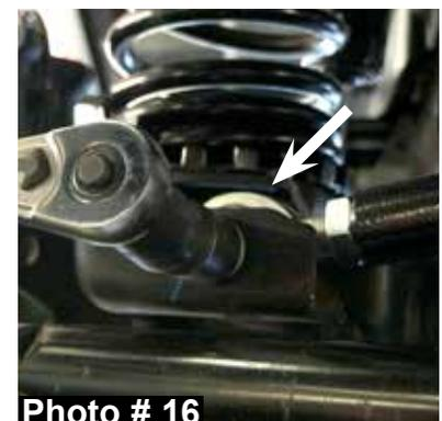
32. Tighten the supplied jam nut of the new Skyjacker adjustable front track bar using a 1-1/8" wrench.
