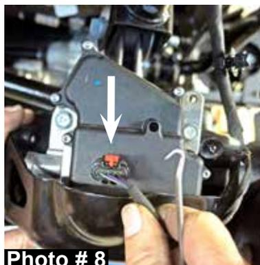
13. Disconnect the OEM vent hose from the front differential using pliers.
