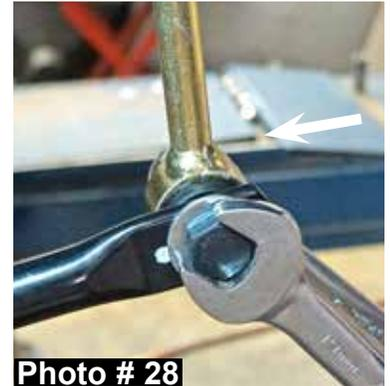
17. Disconnect the OEM rear ABS lines from the OEM rear flex brake lines.
