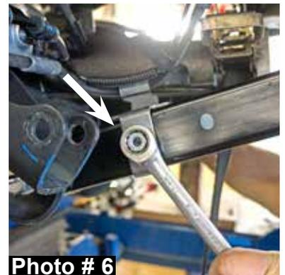
10. Mark the location of the OEM front driveshaft \ flange at the front differential & disconnect using a 15mm socket \ wrench. (See Photo # 7)
