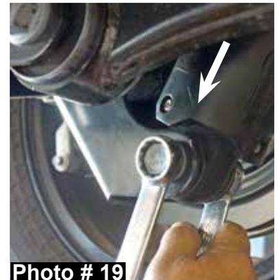
6. One at a time, remove the OEM rear upper control arms & install the new Skyjacker rear upper control arms using the OEM hardware, a 21mm socket \wrench & 24mm socket \wrench. (See Photo # 20)
