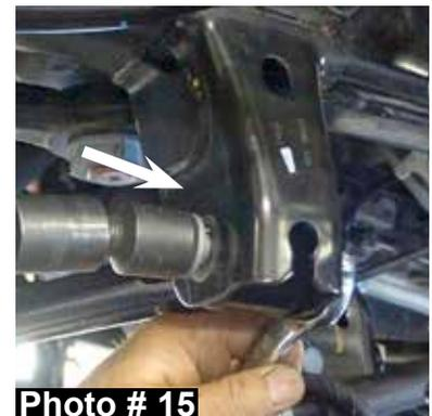
30. Using a measuring tape, check the front of the vehicle to make sure the body is centered over the front tires \ wheels & adjust the new Skyjacker rod end to align with the lower track bar mounting location.
