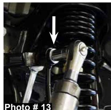
25. Install the new Skyjacker front sway bar end links using the supplied steel sleeves, 12mm x 70mm bolts, 7/16" USS washers, 12mm nuts, OEM hardware, a 18mm socket / wrench, & 19mm socket / wrench. (See Photo # 13) **Note:** On the driver side of the vehicle, install the OEM lower bolt with the large washer to the bushing side of the new front sway bar end link.
