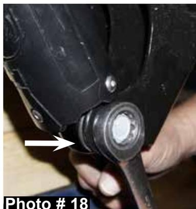
7. Install the new Skyjacker rear bump stop spacers to the OEM rear bump stop pads using the supplied 5/16" x 1" bolts, 5/16" washers, 5/16" nuts, & 1/2" wrenches. (See Photo # 19) **Note:** Install the new rear bump stop spacers with the forward angle toward the front of the vehicle.
