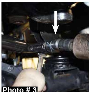
7. Disconnect the OEM drag link from the OEM pitman arm using a 21mm socket / wrench. (See Photo # 4)
