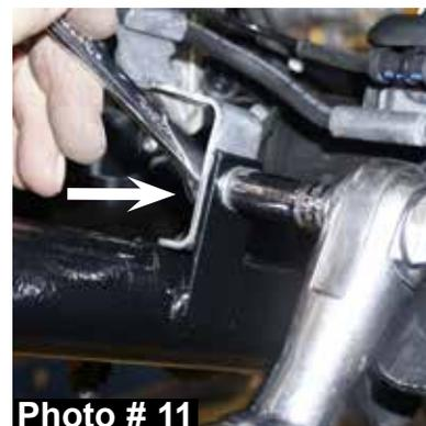
22. One at a time, remove the OEM front lower control arms & install the new Skyjacker front lower control arms using the OEM hardware, a 21mm socket / wrench, & 24mm socket / wrench. **Note:** Install the new front lower control arms with the offset bend toward the inside of the vehicle.
