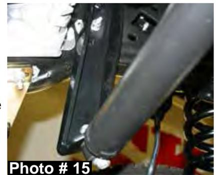
37. **4" Lift:** Install the OEM steering stabilizer to the new Skyjacker frame bracket & OEM drag link using the OEM stud hardware, supplied 12mm x 60mm bolt, washers, nut, a 18mm, & 19mm socket / wrench. (See Photo # 15) **Note:** The OEM steering stabilizer will mount to the bottom side of the new steering stabilizer bracket mounting surface for a 4" lift.
