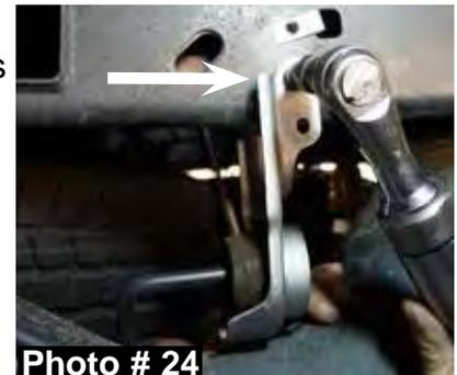
20. Install the new Skyjacker rear shocks using the OEM hardware, supplied hardware, a 18mm, & 21mm socket / wrench.
