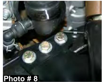
23. Complete the installation of the new Skyjacker track bar bracket to the frame using the OEM hardware, & a 18mm socket / wrench. (See Photo # 9) **Note:** Tighten the new track bar bracket hardware at this time using a 18mm, 13/16", & 7/8" socket / wrench.
