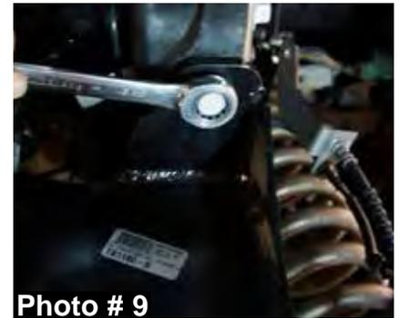
24. Remove the OEM bump stops & bump stop cups from the frame using a 10mm socket / wrench.
