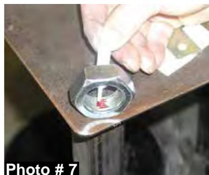
22. Install the new Skyjacker track bar bracket to the OEM location on the cross member using the supplied 9/16" x 3" fine thread bolts, washers, nuts, a 13/16", & 7/8" socket / wrench. **Note:** Use the three .938" long anti-crush spacers between the front of the new track bar bracket & the OEM cross member. Do not tighten at this time. (See Photo # 8)
