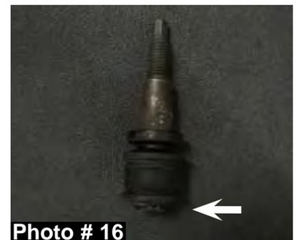
39. **6" Lift:** Remove the OEM tapered stud & bushing from the OEM steering stabilizer using an arbor press. (See Photo # 16)
