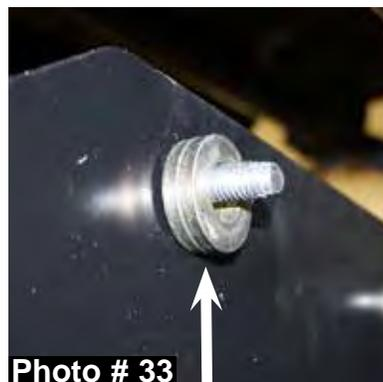
33. Install the new Skyjacker front differential skid plate to the new rear cross member using the supplied 3/8" x 1 1/4" thread cutter bolts & washers. (See Photo # 34)
