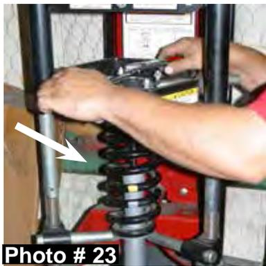
20. Install the OEM coil & top assembly to the new Skyjacker strut.
