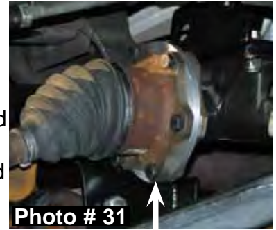
Photo # 31 Passenger side shown with one 15/16" cv-spacer.
